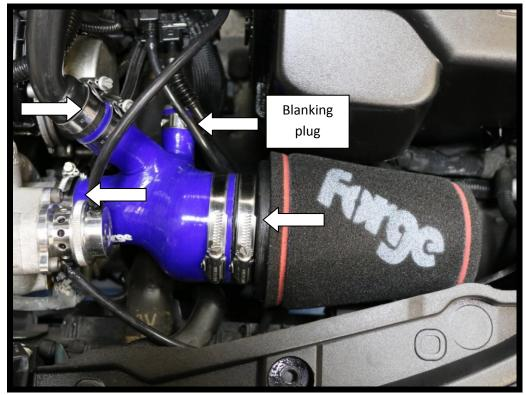
12. For the Citroen DS3 place the intake on the turbo and orientate it so that the pipes on the car line up with the pipes on the intake, then tighten the hose clamp on the turbo. Install the straight joiners and refit oil breather lines.
