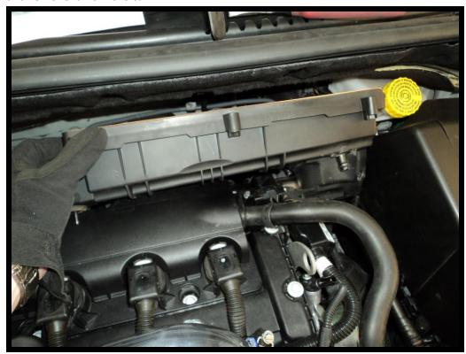
11. For the Peugeot place the intake on the turbo and orientate it so that the pipes on the car line up with the pipes on the intake, then tighten the hose clamp on the turbo. Install the stepped joiner and blanking plug.
