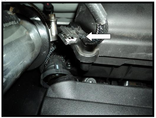
10. Remove the bottom of the air box by pulling upwards to release it from its rubber mounts, and remove it from the car.
