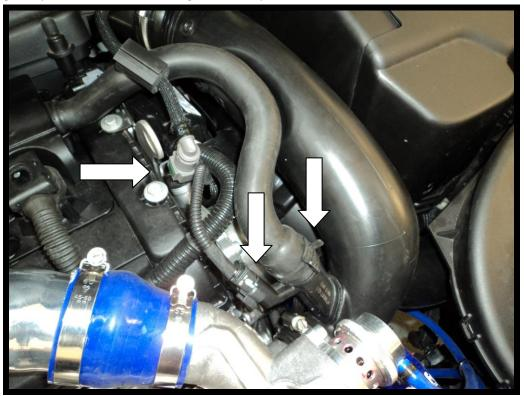
3. Release the secondry breather hose by squeezing the retaining tabs top and bottom and pulling the hose off towards the firewall – this is not on the Peugeot 207. Loosen the hose clip securing the pipe to the turbo with a 7mm hose clamp driver. Remove the turbo to airfilter intake pipe from the car.
