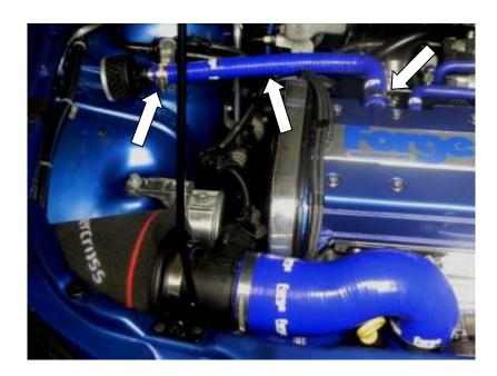
7. Attach the short intake 60-70mm silicon hose to turbo inlet using a suitable jubilee clip. Do not tighten fully as the silicon hose may need to be rotated. Insert MAF sensor into the open end securing its position with a jubilee clip. CHECK THAT THE DIRECTION OF FLOW IS CORRECT (normally shown by an arrow cast into the MAF housing).
