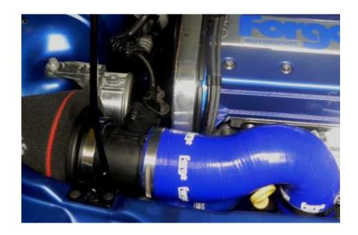
8. Using your remaining jubilee clip, put your new Pipercross filter on the open side of the MAF sensor housing.
