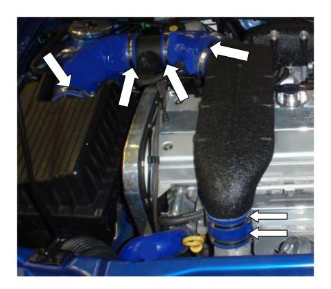
2. Unbolt the oval pipe support bracket using 10mm socket. Using a large set of pliers open the clip on breather hose running to cam cover.
