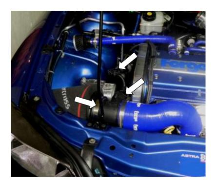
9. Rejoin your MAF to the main vehicle wiring loom using the 200mm 5pin MAF extension loom. Ensure the connectors are firmly pushed together.
