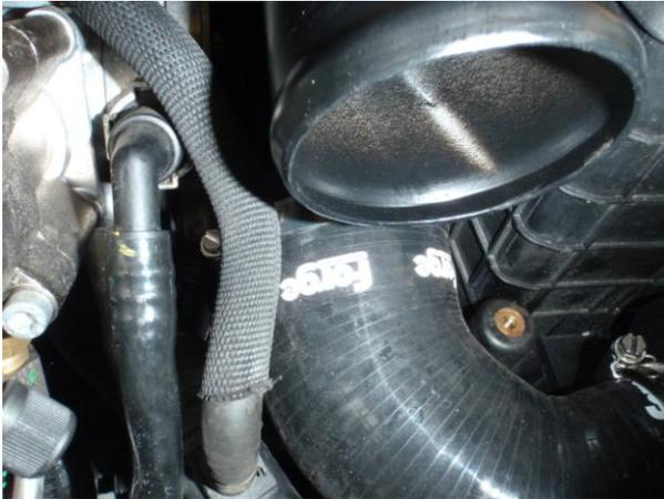
The second hard pipe can now be connected to the turbo inlet pipe using a 70mm silicone coupler. Leave this joint loose initially to allow the positioning of the pipe, allowing equal clearance between the engine and battery.
