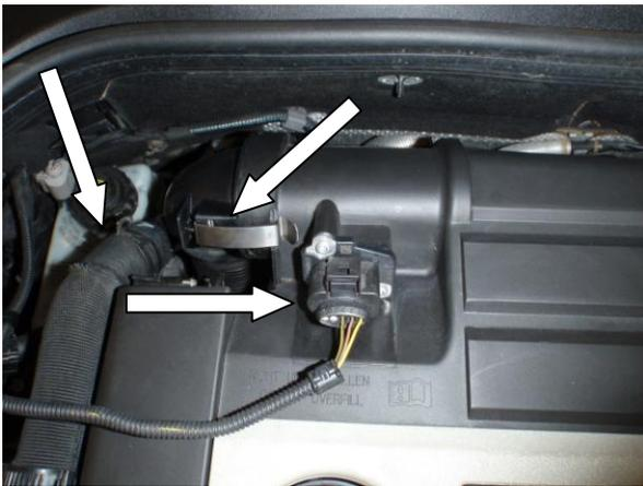
Disconnect the wiring connector to the MAF sensor, then un-clip the turbo inlet pipe from the engine cover .
