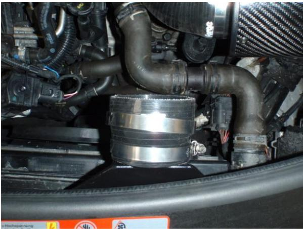
The forward facing ram-air duct is now attached to the front radiator support / slam panel using the original T25 Torx screws that secured the original intake ducting that were removed previously.
