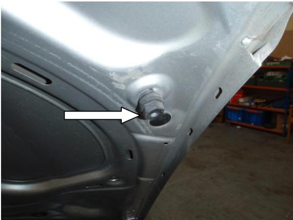
When closing the bonnet/ hood for the first time, check the level of the panel against the wing / fender edge. If necessary adjustment can be made with the adjusters found on the underside of the bonnet / hood as indicated.
