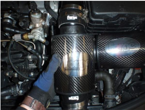
You can now attach the second carbon canister using the remaining two 76-70 straight couplers. Due to the fixed nature of the pipe and the forward ram-air inlet duct, it will take some effort and maneuvering to insert the canister and attach both couplers to the piping. Once both couplers are attached to the piping, however, secure the hose clamps.
