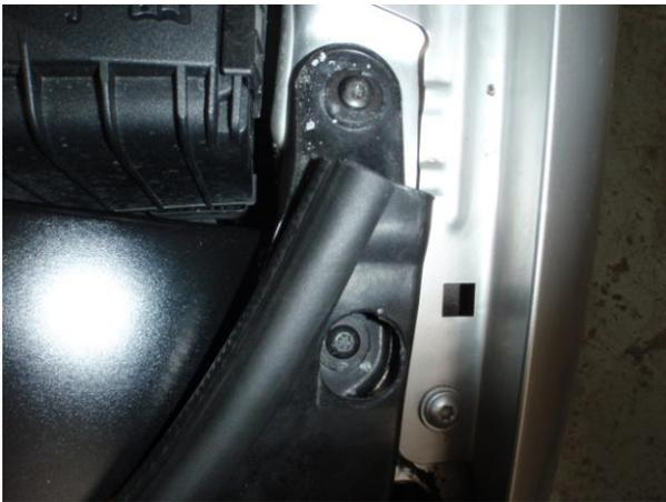
You now need to attach the two inlet ducts. The side duct is secured using the two T30 Torx screws that secure the upper edge of the radiator support just behind the headlight.
