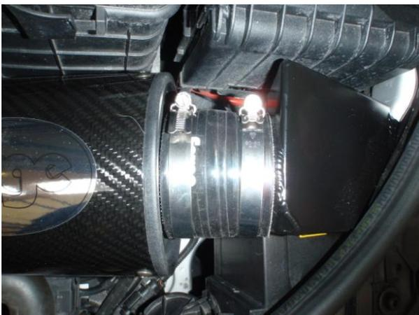
You may find it easy to attach one of the carbon filter canisters at the same time, using a 76-70 straight coupler hose to attach the opposite end of the filter canister to side inlet duct, securing it with a #90 and #80 hose clamp. NOTE: During installation, the filter canisters should be oriented so that the the open end of the filter is attached to the pipework going to the throttle body and the pointed end of the filter is attached to the inlet duct.
