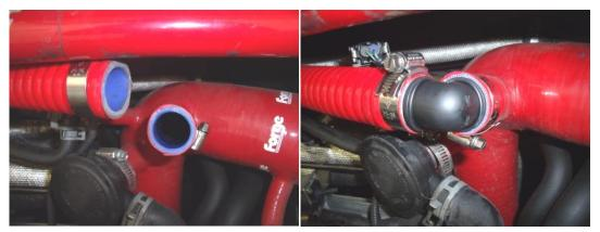
• Using the vacuum tube supplied relocate the vacuum line across the top of the inlet manifold and clip up tight with the cable ties supplied, Fit to the dump valve again using a cable tie.
