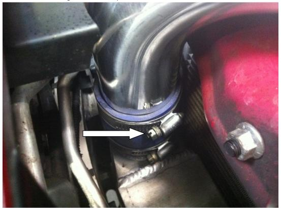
12. Tighten the support hose clamp using a flat headed screw driver.
