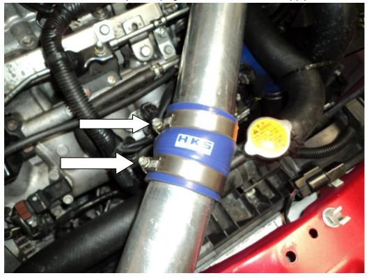
5. Undo this hose clamp situated closest to the turbo, using a flat headed screwdriver.
