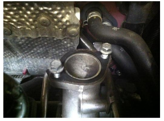
9. Now slide the new Forge aluminium billet outlet flange onto the two 12mm bolts sitting on the turbo housing, again making sure you don't damage the gasket. When fitting this please make sure the vacuum pipe is situated on the top right hand side as your looking from the front of the vehicle. Tighten the two 12mm bolts.
