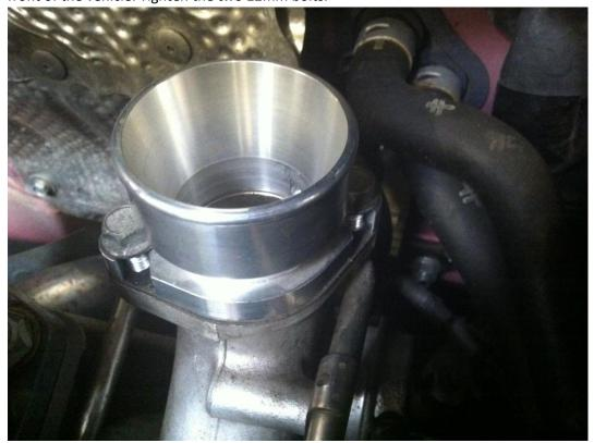
10. Now place the new forge silicon hose over the Forge aluminium billet outlet flange and secure at the bottom with a hose clamp provided. Once the hose is tightened to the flange, you can now fit the new forge aluminium boost pipe into the forge silicon hose and tighten with a hose clamp provided.
