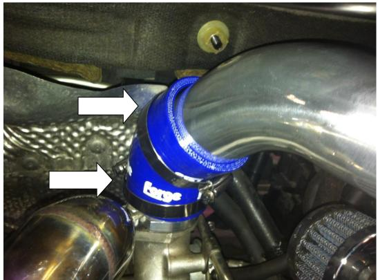
11. Now fit the other end of the forge aluminium boost pipe into the silicon hose on the top of the intercooler and tighten hose clamp.
