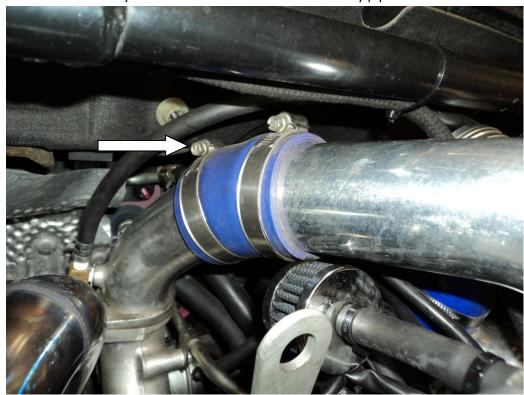
6. Now you will have to remove the silicon pipe that goes onto the take off in the picture shown below. To remove this simply clamp the two tabs together and pull the pipe off.
