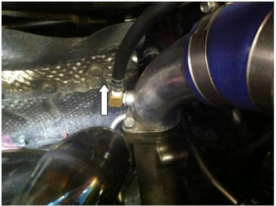
7. Using a 12mm spanner under the two 12mm bolts holding the aluminium flange to the turbo housing and then remove it. Make sure you don't damage the gasket when taking this off
