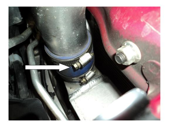
3. Undo the hose clamp using a flat headed screw driver to release the alloy pipe from the clamp.
