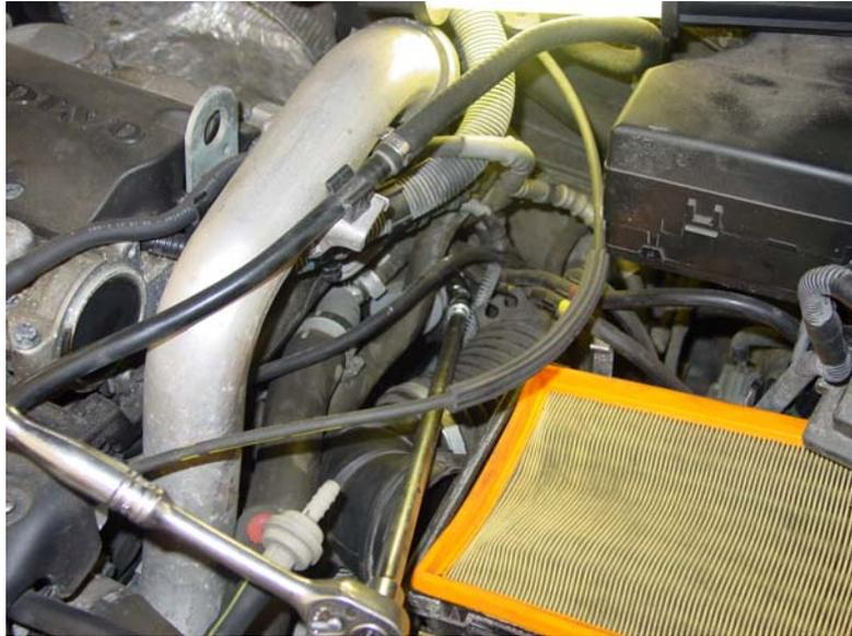
If you move some of the intake and coolant hoses to the side gently you can gain access to the 3x10mm bolts that secure the diverter valve. Firstly remove the vacuum hose to the valve; there will be a small clip which can be removed simply with a pair of pliers. Then remove the 3x10mm bolts (these are tricky to get to so a knuckle joint and extension will be required as pictured above. Remove the complete valve (as below picture and then fit the new blank plate in to this position.
