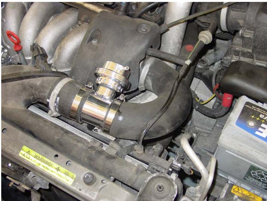
2/ Remove the air box lid as shown below in order to gain access to the original diverter valve located in the side of the turbo housing.
