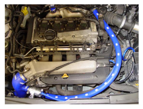
1/ Open bonnet/hood. Remove the plastic engine cover. Remove the hose running between the throttle body housing and the top intercooler connection (bottom left hand corner of the picture above)
