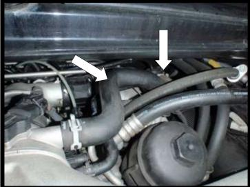
1. Remove the OEM valves and rubber hoses, using blanking plugs supplied in kit, blank off the holes in the intakes. Install the silicon hoses and dump valves to the Y pipe and your installation is complete.
