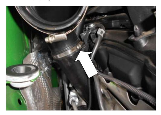
7. Using a 6mm hose clamp driver undo the 2x hose clamps and pull the OEM hoses off of the chargecooler inlet pipes.
