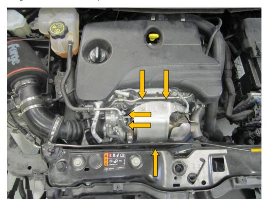
2. Remove the turnbuckle from the oem actuator and transfer it to the Forge Motorsport actuator without fully tightening the lock nut.
