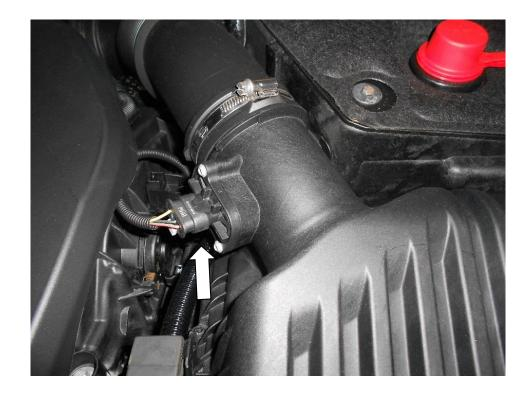
4. Using a 7mm Hose clamp driver or flat blade screwdriver undo the hose clamp.
