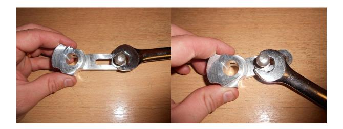
12. Secure your Forge quickshifter in position using the split pin supplied. Ensure the up and down shift arm is correctly located. Start the split pin off the car on a solid surface before fitting in to the gearbox shaft.
