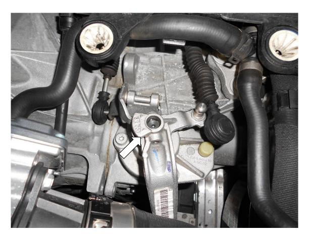
11. Using a 16mm spanner tighten the adjustable ball in the required position. Closer to the pivot will give a shorter shift and further away will give a longer shift. Set the adjuster at the midway position.
