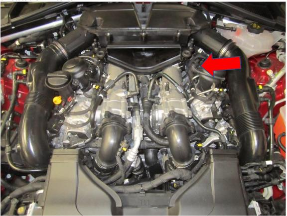
4. Using an m6 Allen key remove the map sensor from situ.
