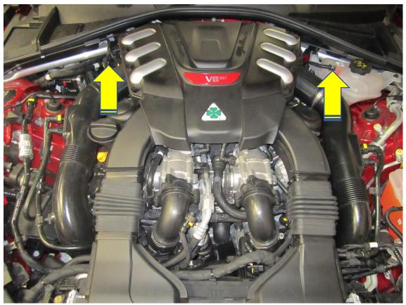
2. Remove the two rubber inlet hoses along with the intake scoop again by pulling sharply in an upwards motion.
