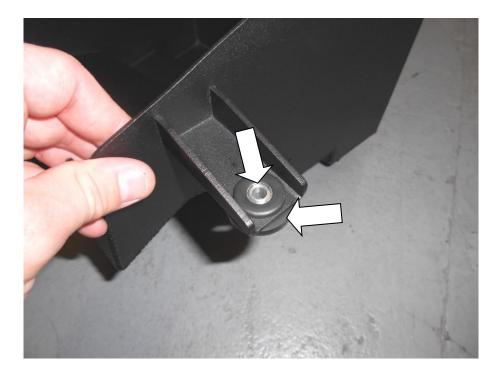
11. Carefully fit the airfilter tray in position and secure with the M6x20mm Allen bolt and 6mm penny washer.
