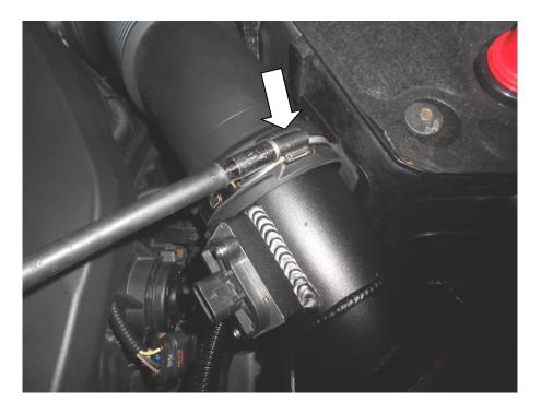
15. Reconnect the wiring to the MAF sensor.
