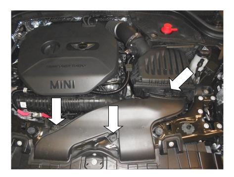
3. Carefully disconnect the wiring to the sensor on the intake.
