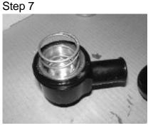
Check that the piston travels freely within the body of the valve before screwing the top back on.
