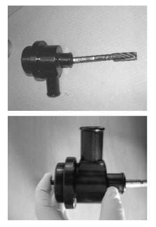
A simple test that you can perform on your valve is to use a pen and push the piston of the valve upwards against the spring to ensure that it moves without restriction. Then with the piston pushed fully up, ie with the spring compressed, place your finger over the top nipple to form a seal.
