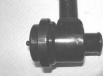
To remove the top of the valve carefully unscrew the top.
