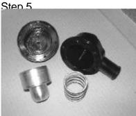
With the disassembly completed, wipe all the components clean with a soft tissue or cloth
