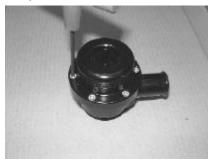
Carefully remove the Allen Cap screws - be aware that the top will spring apart if not restrained
