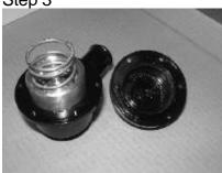
With the top removed you can remove the spring and piston from the valve body and .....
