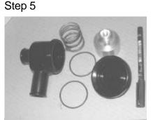
Dis-assembly complete. Carefully clean all the parts with soft tissue or cloth
