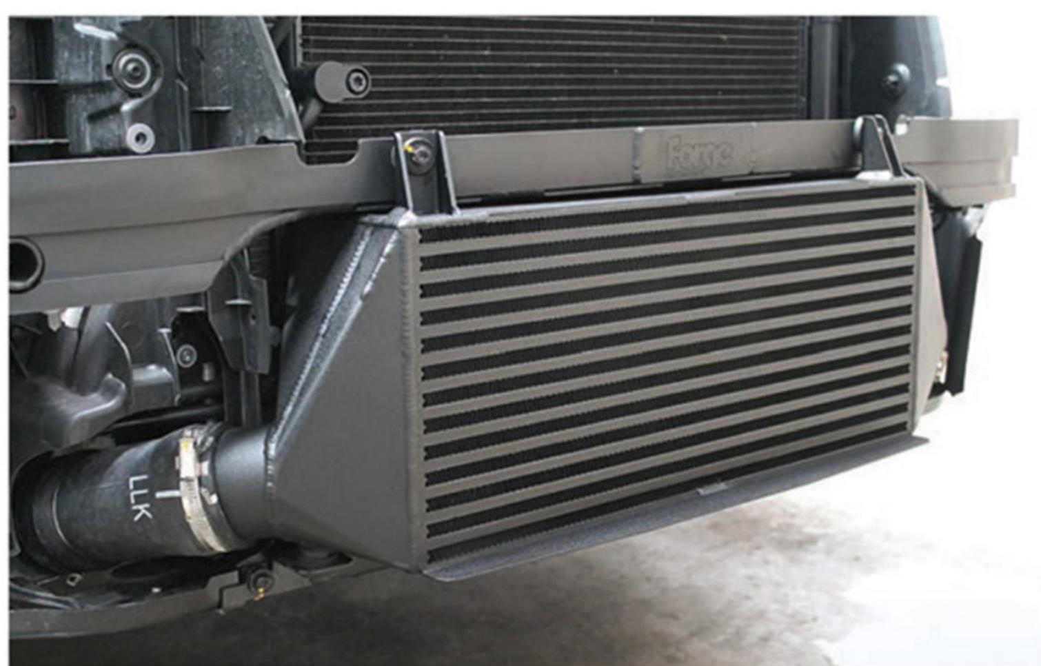
'Forge Motorsport seized the opportunity to design a much larger intercooler core to provide more surface area and cooling efficiency than the stock intercooler, with the number plate repositioned to provide maximum airflow through the grille...'
