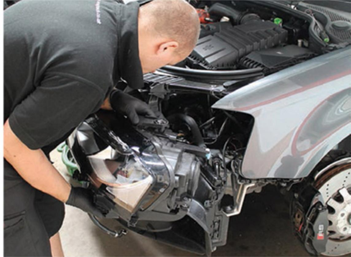
for the RS 3, one which didn't involve any external bodywork modifications. Indeed, it was almost a straightforward bolt-on conversion. It seems that there's a huge amount of space between the radiator and the inside of the front bumper, but that the Audi engineers had seen fit to install only a fairly modestly sized intercooler as standard.
