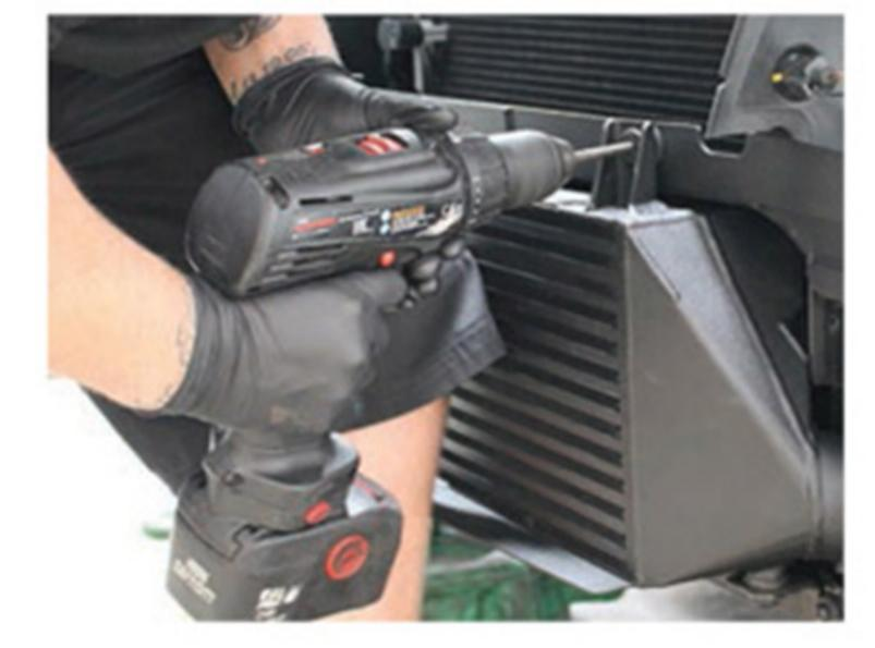
aluminium sleeves fitted into the top brackets, and the drill bit supplied in the kit is used to drill perfectly positioned holes to attach the intercooler accurately at the top.
