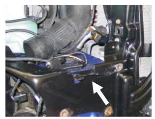
On the front panel of the vehicle, bend down the optional headlight washer bracket as shown
