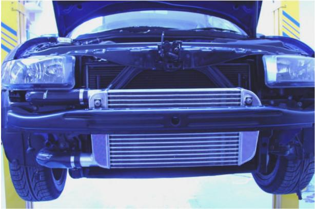
On refitting the front plastic over bumper it will be necessary to trim the plastic internal webbing on the inside of the bumper near to where the towing eye is located. This is to allow clearance for the lower intercooler hose.
