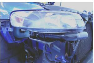
Install the new hose to the intake manifold and reconnect the MAP sensor electrical connector. Now refit the headlight along with its four securing bolts and electrical connector
