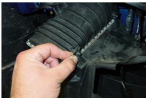
Unclip and remove the air guide from the front of the intercooler
