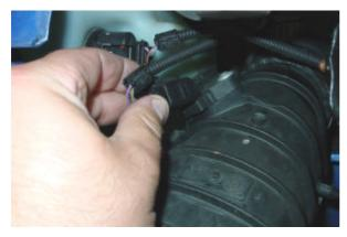
Disconnect the electrical connector to the (MAP) pressure sensor on the existing intercooler if fitted.
