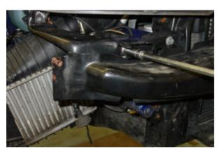
Remove the bolts from the metal crash bumper each side of the vehicle and remove the bumper
