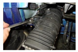
Remove the intercooler mounting bolts and remove the intercooler
