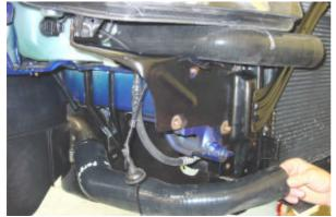
Install the lower intercooler hose as shown
