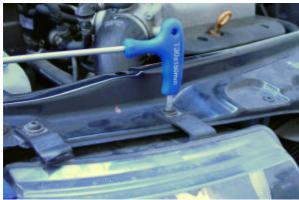
Remove the two upper and two lover torx bolts from the headlight unit on the intercooler side of the vehicle. Disconnect the electrical connector and remove the headlight unit.
