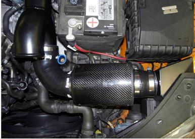
You will now attach the second carbon cannister to the upper split in the pipe using the remaining two 76-70 straight couplers. Due to the fixed nature of the pipe and the forward ram-air inlet scoop, it will take some effort and manuevering to insert the cannister and attach both couplers to the piping. Once both couplers are attached to the piping, however, loosely secure the hose clamps.
