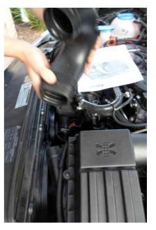
At the rear of the airbox just is a 5mm Allen Bolt. Unscrew this bolt and also release the metal clamp at the rear of the MAF housing. This will allow you to lift the entire airbox and MAF housing assembly out of the engine bay. It is secured in place by some rubber grommets, but these are easily overcome with a little force.
