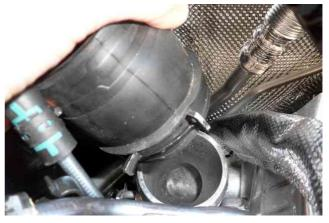
You will now need to attach the two inlet scoops to the front end of the car. The forward facing ram-air duct will be attached to the front radiator support / slam panel using the original T25 Torx screws that were removed previously that secured the original intake ducting.
