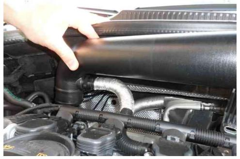
Next, you will remove the rubber coupler at the turbo inlet. Using your pliers, remove the last pinch clamp to release the rubber coupler and remove it.
