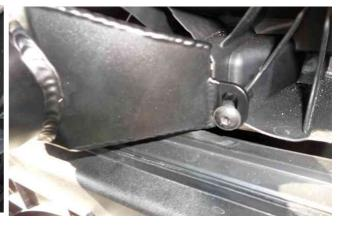
The side inlet scoop is secured using either 1 or 2x T30 Torx screws that secure the upper edge of the radiator support and/or headlight. This will be unique to each vehicle application. Shown below are a few examples.
