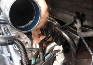
Follow the hard plastic intake tube to the left to the turbo inlet. At the bottom will be two metal pinch clamps and a rubber hose coupler. Using your pliers, release the upper pinch clamp and pull the plastic tube up. This will expose the small corrugated rear PCV tube that is clipped to the intake pipe. Using a flathead screwdriver, VERY CAREFULLY release this clip connection to disconnect this tube and be careful not to break the clips.
