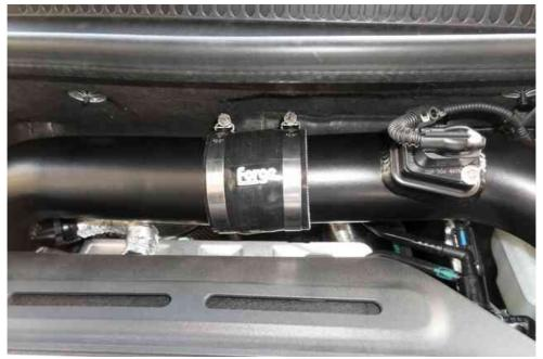
You will now attach the 90 degree reducing elbow hose to the lower split of the "Y" pipe. The smaller 70mm end will attach to the pipe while the larger 76mm end will point towards the side inlet scoop. You may wish to remove the battery cover for easier access to attach the hose and secure it to the pipe with a #80 hose clamp.
