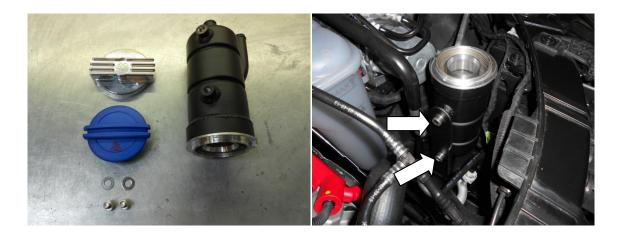
32. Slide the Forge billet expansion tank cover over the top of the OEM VAG Expansion cap and secure with grub screw.
