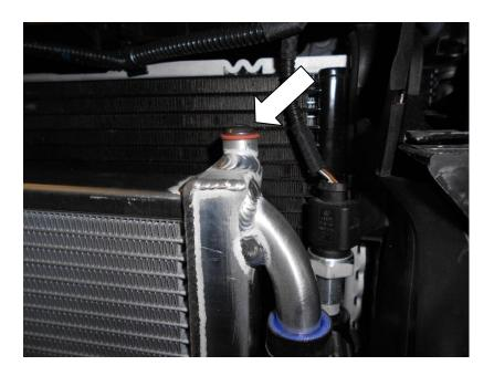
39. Check the silicone hoses for any signs of leaks before replacing the bumper.
