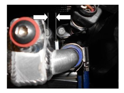
23. Using a rule and fine liner pen mark the position of the R/H bracket on the crash bar.
