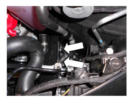
29. Using 10mm spanner undo nut and remove A/C pipe bracket.
