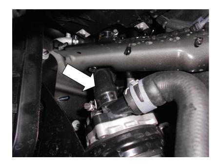
34. Join the lower radiator outlet silicone hose (which should already be attached to the radiator) to the side pipe on the expansion tank and secure with a suitable hose clip.
