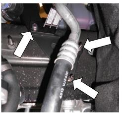
31. Using the 2x M8x12mm Allen cap bolts and M8 washer attach the Forge expansion tank to the bracket.
