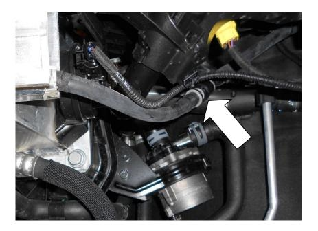
19. Moving to the other end of the crash bar disconnect the other end of the washer hose.
