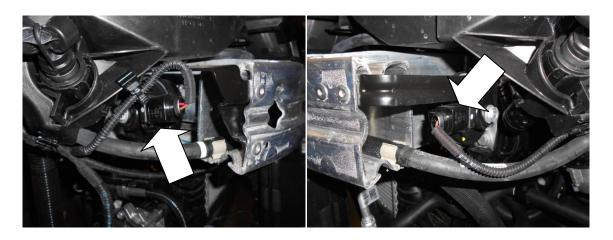
18. Disconnect the headlight washer tube and drain the remaining washer fluid into a suitable container. This will need to be replaced when the installation is complete.
