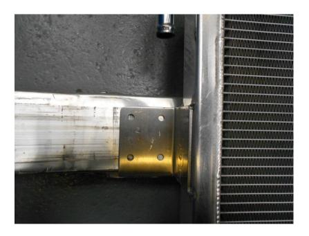
26. While the crash bar and radiator are off the vehicle fit the lower charge cooler radiator silicone hose, with suitable hose clip. Secure the 28mm P-clip with the M6X12m Allen cap bolt and washer provided.
