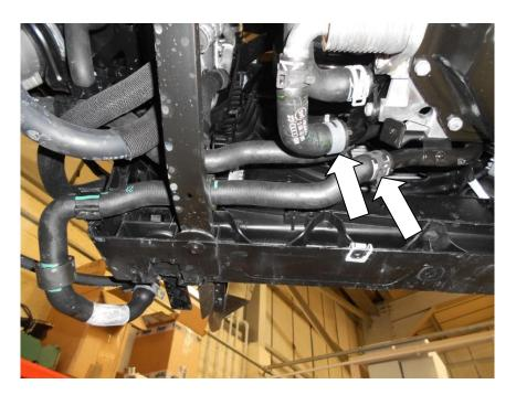
B) 2x Hoses on the pump inlet and outlet.
