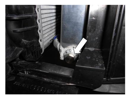
38. Undo the bleed screw located on the top R/H side of the charge cooler radiator. Fill the expansion tank with coolant until the coolant starts to appear at the bleed hole, then refit the bleed screw and sealing washer.
