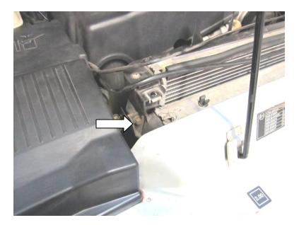
Undo the 10mm intercooler to radiator bolt
