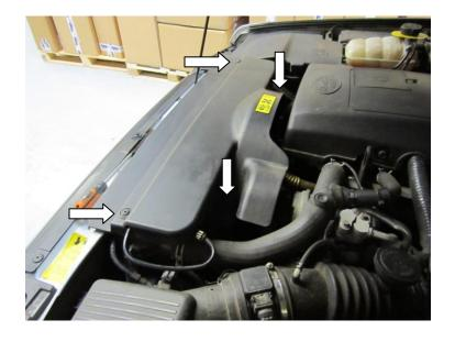
Unscrew the four Philips head screws half a turn anticlockwise.
