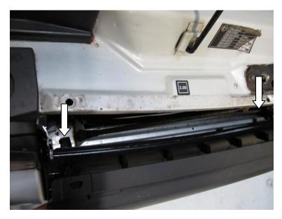
Pull the Grille towards you then pull upwards to release the grille from the vehicle.
