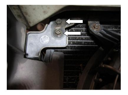
Undo the two 10mm air conditioning radiator bracket bolts, and remove the bracket from the vehicle.
