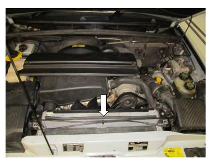
Using the supplied cable tie secure the two plastic pipes together.
