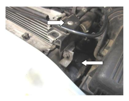
Remove the two intercooler hoses by undoing the hose clamp using a flat head screwdriver or a 7mm hose clamp driver.
