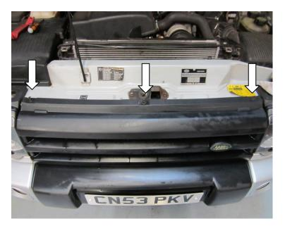
Unscrew the three plastic Philips head screw clips from the plastic clip insert.
