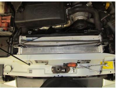
Fit the Forge intercooler again you will need to lower the driver's side in first (RHD car).
