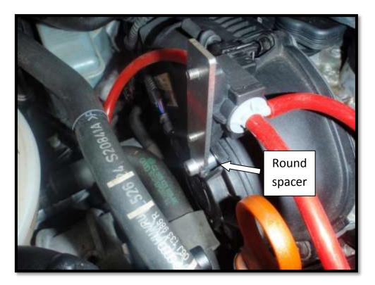
5. Remove the Plastic boost pipe by removing the hose clamps the 10mm nut and the T30 torx that secures the pipe to the engine block this can be tricky due to limited space. You will need to remove the under tray to access the T30 torx.
