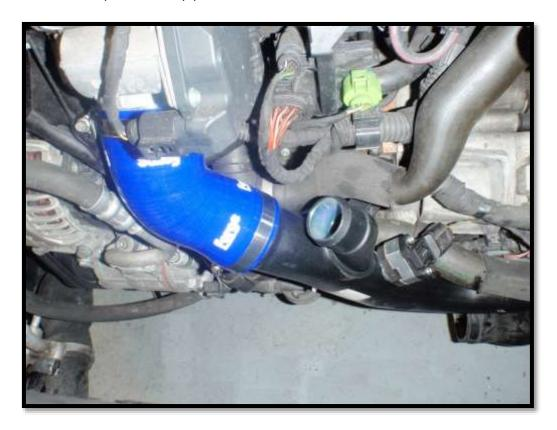
8. Install the silicone hose and BOV with the clips supplied in kit.
