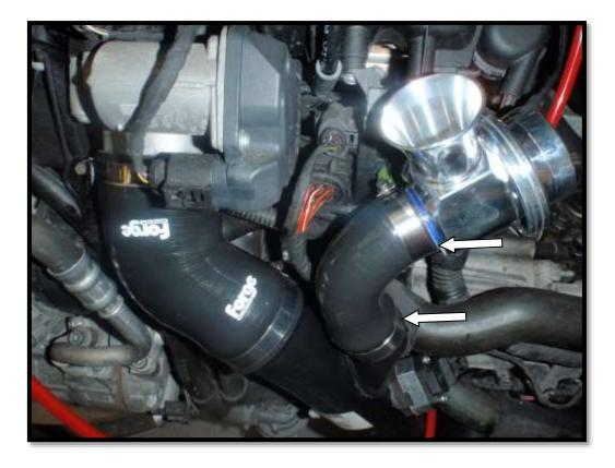
9. The photo below shows how to install the vacuum hoses and wiring extension.
