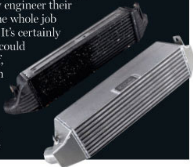
Below Forge i/c is much thicker than OEM unit
