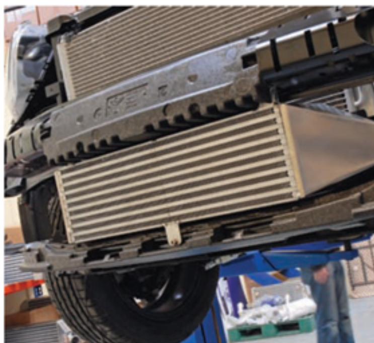
Countryman's front end offers more space than the MINI hatch for the intercooler.
