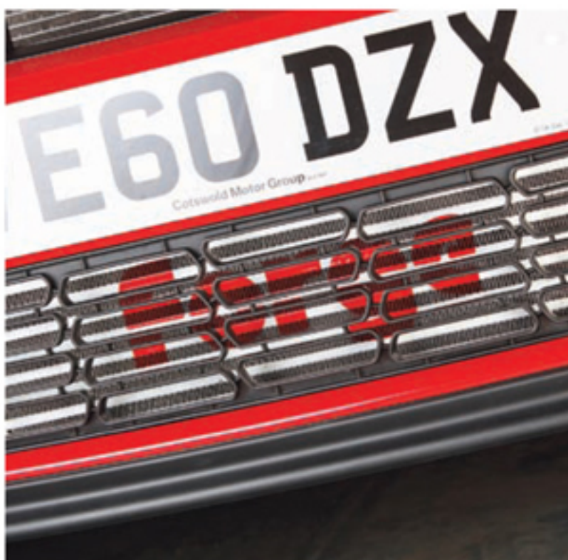
Above: Forge intercooler fits without bodywork alterations.
