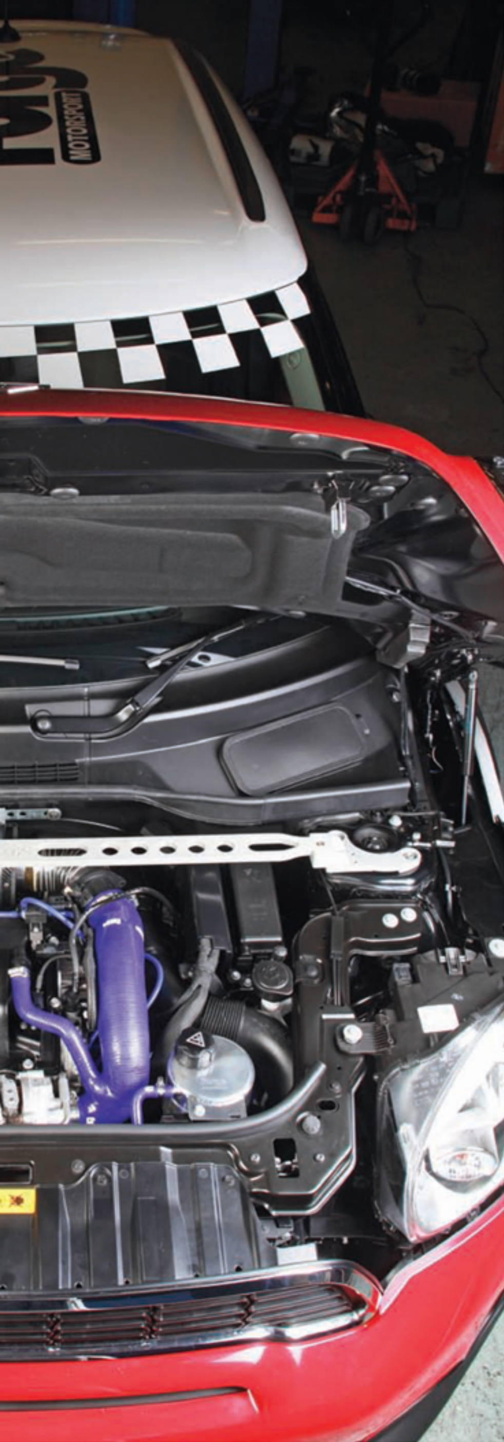
Left: Engine spec includes uprated induction, Forge blow-off valve and silicone hose kit. And not forgetting the trademark alloy header tank.
