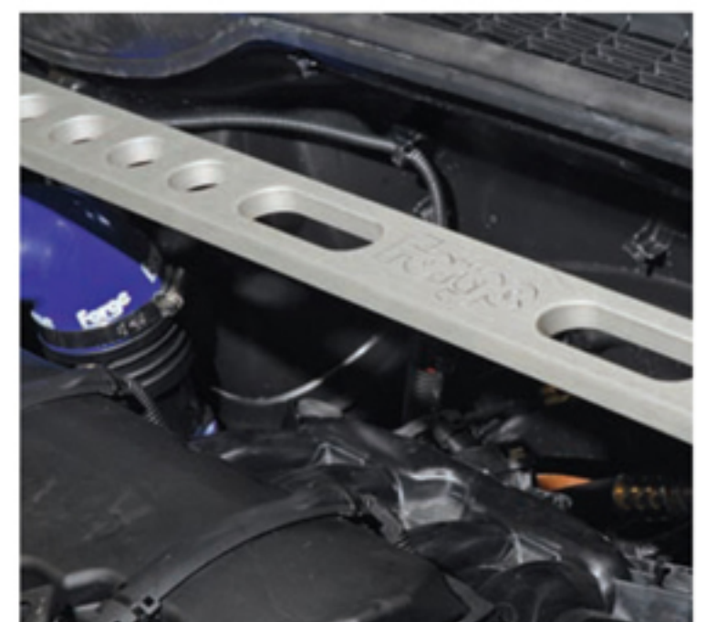
Prototyping the strut brace showed just how much wider the Countryman is than the hatch.
