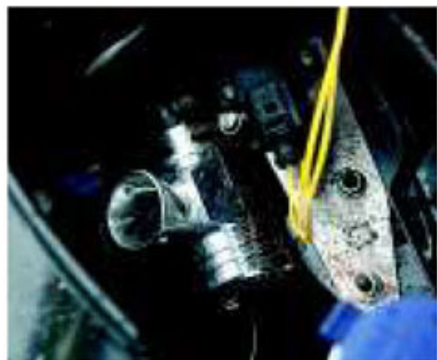
Left Obligatory vent to atmosphere alloy dump valve turns heads
