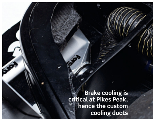
Hiding behind the BBS 'show' wheels are F1 carbon brakes!
